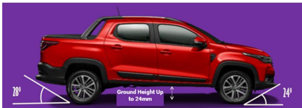
Figure 6. Strada approach angles, departure, and ground clearance [2].
