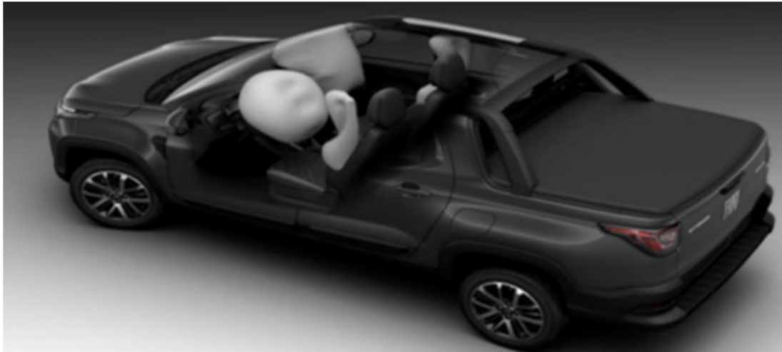
Figure 7. Air bags and internal part of the FIAT Strada [2].
